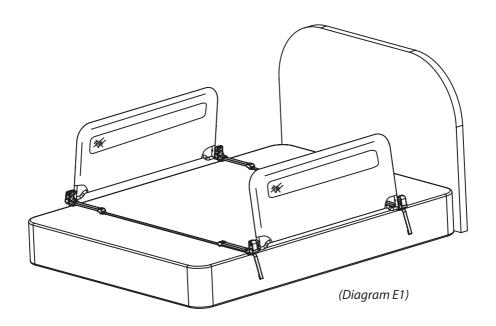
**Step 2:** Once the bed rail is placed properly, place the mattress back atop of the box spring or mattress support sandwiching the flat metal bars of the corner hinges and the anchoring straps between the box spring and the mattress.
